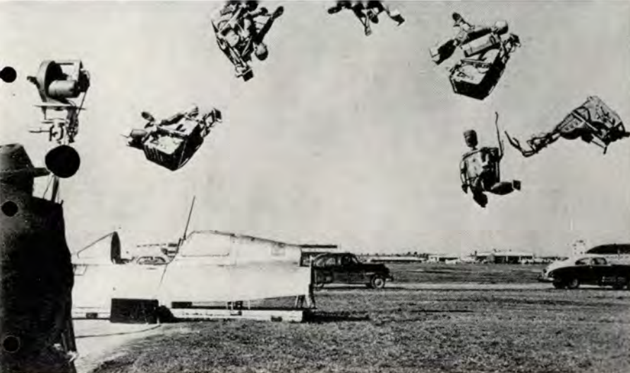
Tests have been made to study the trajectory of seats. When chute is equipped with an automatic opening device and an automatic lap belt, you do nothing but fire the seat.
